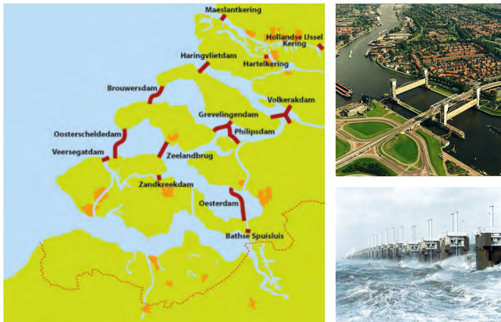
Figure 1: The Delta Works, a €5 billion, 30-year programme of flood defences consisting of levees, dikes, dams, sluices and storm surge barriers. Many new structures were built, together with reinforcement / upgrade of existing defences. a) map of Delta Works. b) 1958 – storm surge barrier in the river Hollandse IJssel. c) 1986 – storm surge barrier in Eastern Schelde. (Source: Rijkswaterstaat via 5 )
